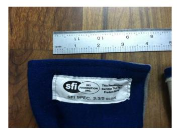
Counterfeit SFI 3.2A/1 Label (incorrect font and different material) on Shayan/FNX single layer suit (photo shows test swatches cut from suit):
